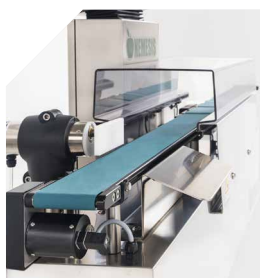
Protective tunnel Essential for compliance with GMP standards in the pharmaceutical industry, it ensures hygiene and safety.
