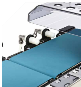
Single or double air-jet ejector Ideal for rejecting light or delicate products.
